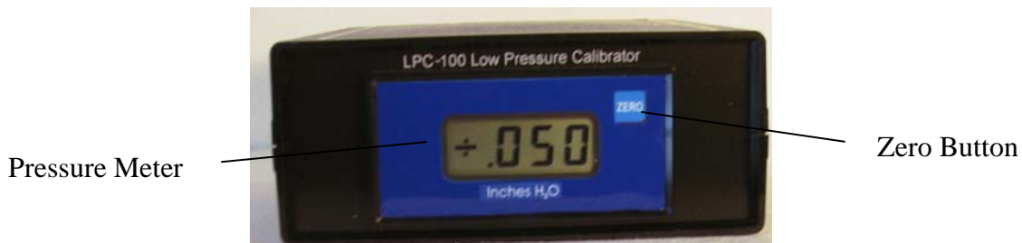
Figure 1. LPC-100 Front Panel
